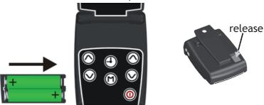
The latch to release the battery compartment can be found on the rear side of the device. Press your finger on the latch until the compartment is ejected.
