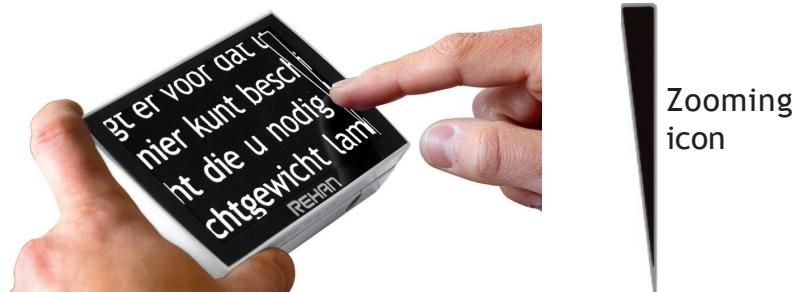
To zoom in slide your finger upwards on the zooming icon, to zoom out, slide downwards on the zooming icon. The magnification range of the Looky 5 ranges from 2x to a 20x magnification.
